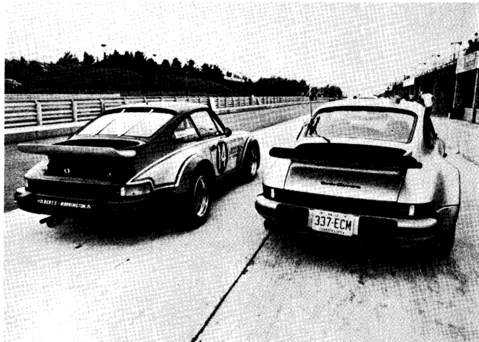
Pop-rieveted fender flares and 16-in. diameter BBS wheels are used on Group 4 Turbo (above left). Specially crafted wrap-around fenders and custom-built 19-in. diameter magnesium wheels are used at the rear of the Group 5 car. Scoop in rear fender (left) directs air to intercooler radiators. Street Turbo and Group 4 car are similar in appearance.
