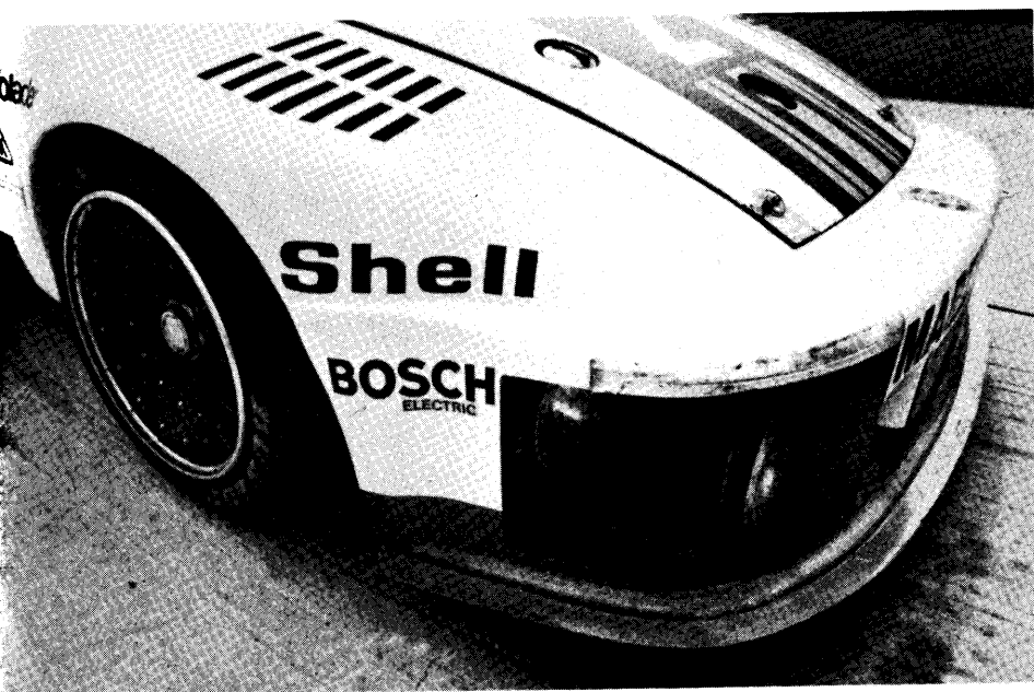
Group 4 car's chin spoiler hides brake ducts and oil and water coolers, but Group 5's is part of 1-piece nose and covers repositioned headlights and oil cooler.
